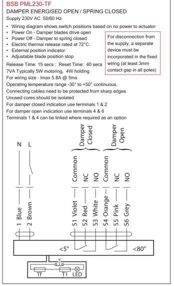
Where the manual adjustment is required and fitted, open indication to be provided by contacts 1 and 3.
