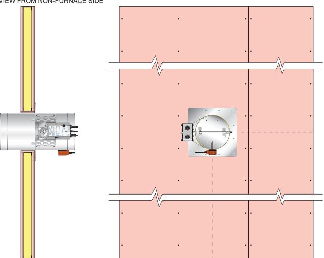
The FSD-C single blade combination fire and smoke damper with its unique feature of requiring only a single installation plate when being installed within tested applications, and without the need for any infill between the damper body and the structure that it sits within. Is the first damper of its type to achieve and exceed the requirements of classification EN1366-2.
