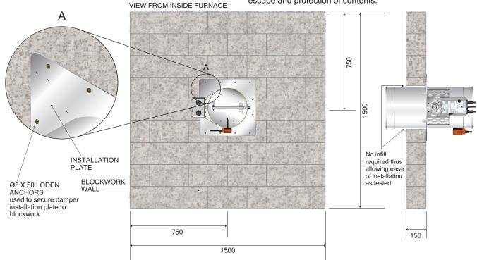
The addition of the PML actuator allows this tested product to become fully automatic in its operation via the fire detection system or one of the BSB control panels. To comply with the forthcoming revision of the fire damper test standard.
