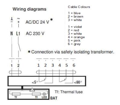
9.5 Make the following connections to achieve indication. closed indication – use 1 & 2. open indication when not using set point positions 4 & 6. open indication when using set point positions 1 & 3
