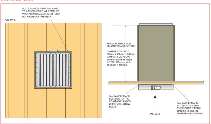
The bulkhead and deck to be in accordance with FTP code 2010 Figure 12. Insulation material and thickness for the bulkhead and deck should be in accordance with the manufacturers instruction. The length specified is required to achieve A60 classification. For AO classification, insulation is not a requirement.
